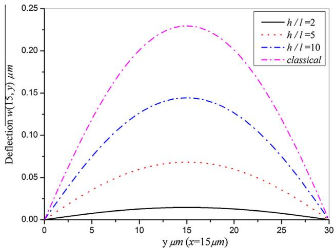
Fig. 3. The deflection distribution on the center section of  $x = 15 \mu\text{m}$ .
