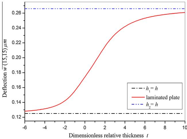
Fig. 2. The deflection at central point varying with dimensionless relative thickness.
