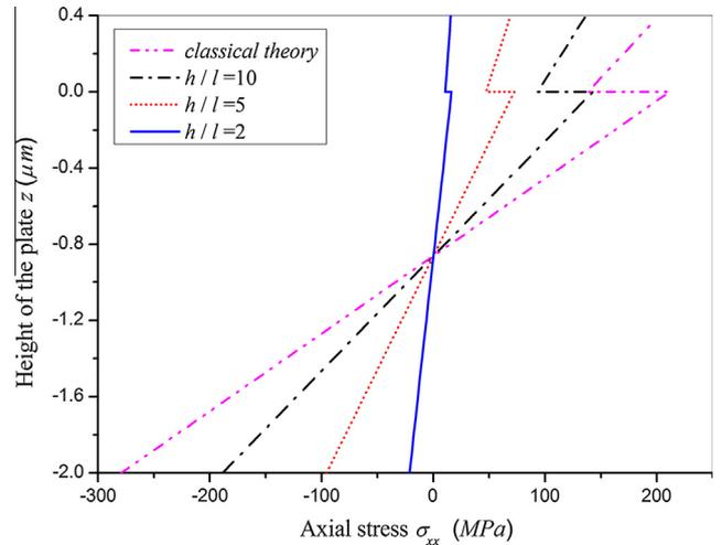
Fig. 5. The distribution of axial stress  $\sigma_{xx}$  along the thickness of plate at central point.
