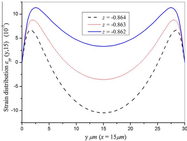
Fig. 7. Distribution of axial strain  $\varepsilon_{yy}$  near the zero-strain surface on the center section of  $x = 15 \mu\text{m}$ .
