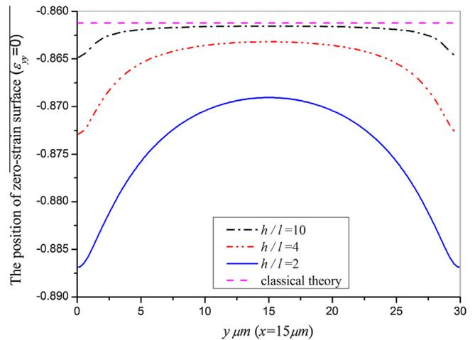
Fig. 6. The location of zero-strain surface on the center section of  $x = 15 \mu\text{m}$ .
