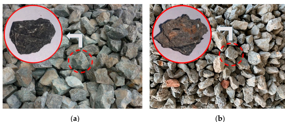
Figure 2. (a) Natural aggregate concrete (NCA) and (b) recycled coarse aggregate (RCA) were used in the experiment.
