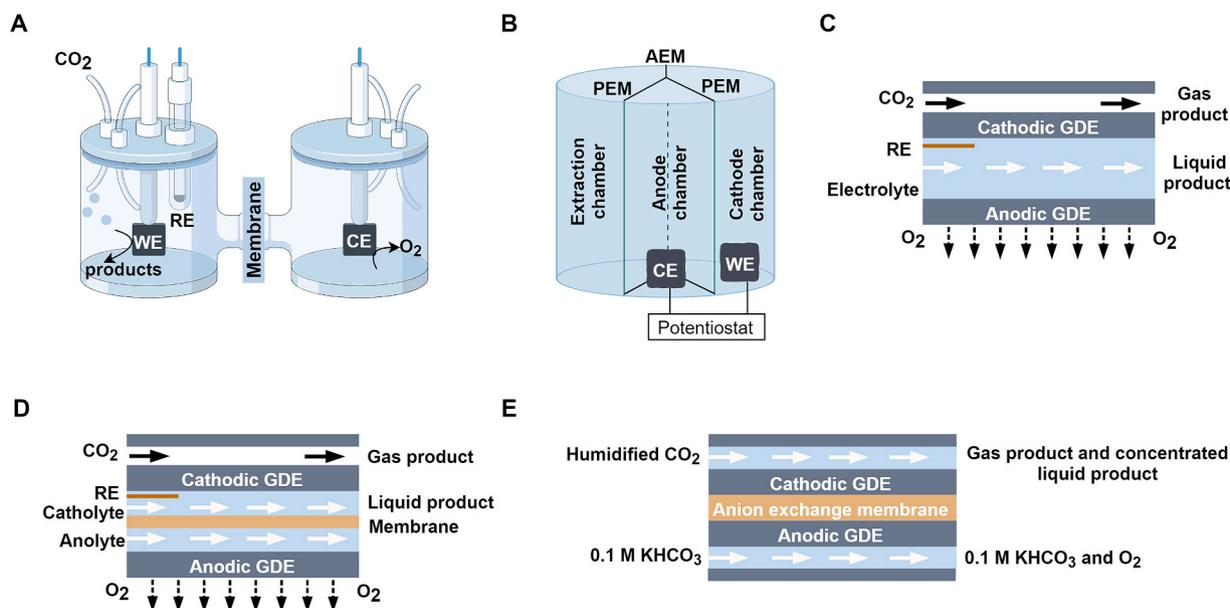
**Fig. 7.** Schematic diagram of different electrocatalytic CO<sub>2</sub> reduction reaction reactors. A: H-shaped reactor. WE, working electrode; CE, counter electrode; RE, reference electrode. B: Triple chamber circular reactor. AEM, anion exchange membrane; PEM, proton exchange membrane. C: Microfluidic reactor. D: Membrane-based reactor. E: Membrane electrode assembly reactors.
